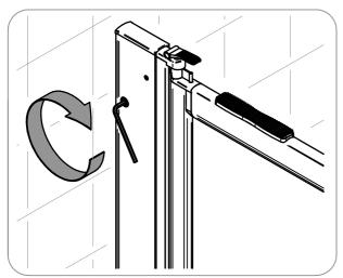
Once the doors are correctly aligned, tighten the upper and lower hex screws with the allen key provided.
