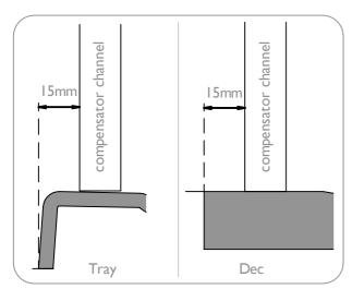
Position the compensator channel 15mm inboard from the edge of the tray/dec as shown.
