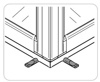
Allow doors to rest on door setters as shown. This ensures the doors are correctly height adjusted.
