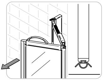
Test the door operation to ensure the doors meet and the floor seal does not drag.
