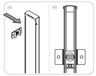
(a) Clip the two plastic locating plates in place. (b) Align the spirit level bubble.
