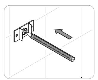
6 Unclip the marking plate and align with the previously marked points. Mark the centre hole for drilling. **DO NOT DRILL OUTER POINTS**
