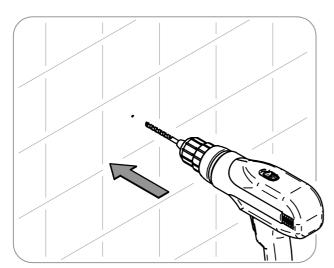
Using a suitable drill bit, drill the upper and lower marked centre points.
