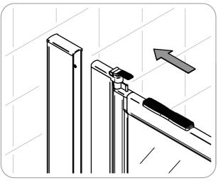
9 Insert the door into the wall compensator.
