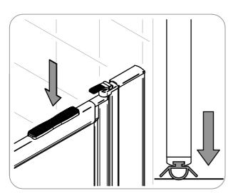
Press down on the push pad to latch the door in the down position again.
