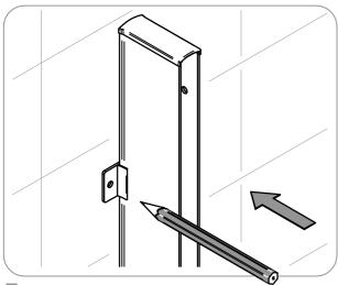
Mark the two alignment points, repeat for the lower fixing. **DO NOT DRILL MARKINGS**
