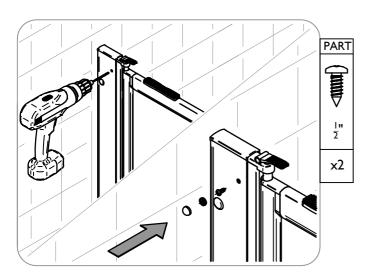
25 Drill (using a 3.5mm bit) and screw lockup holes (x2) in wall side door compensator.
