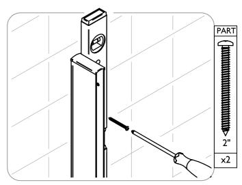
Using appropriate fixings, screw the wall channel into position, ensuring the channel remains vertical.
